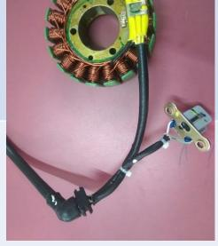
**Stator Wiring Harness Magneto**
